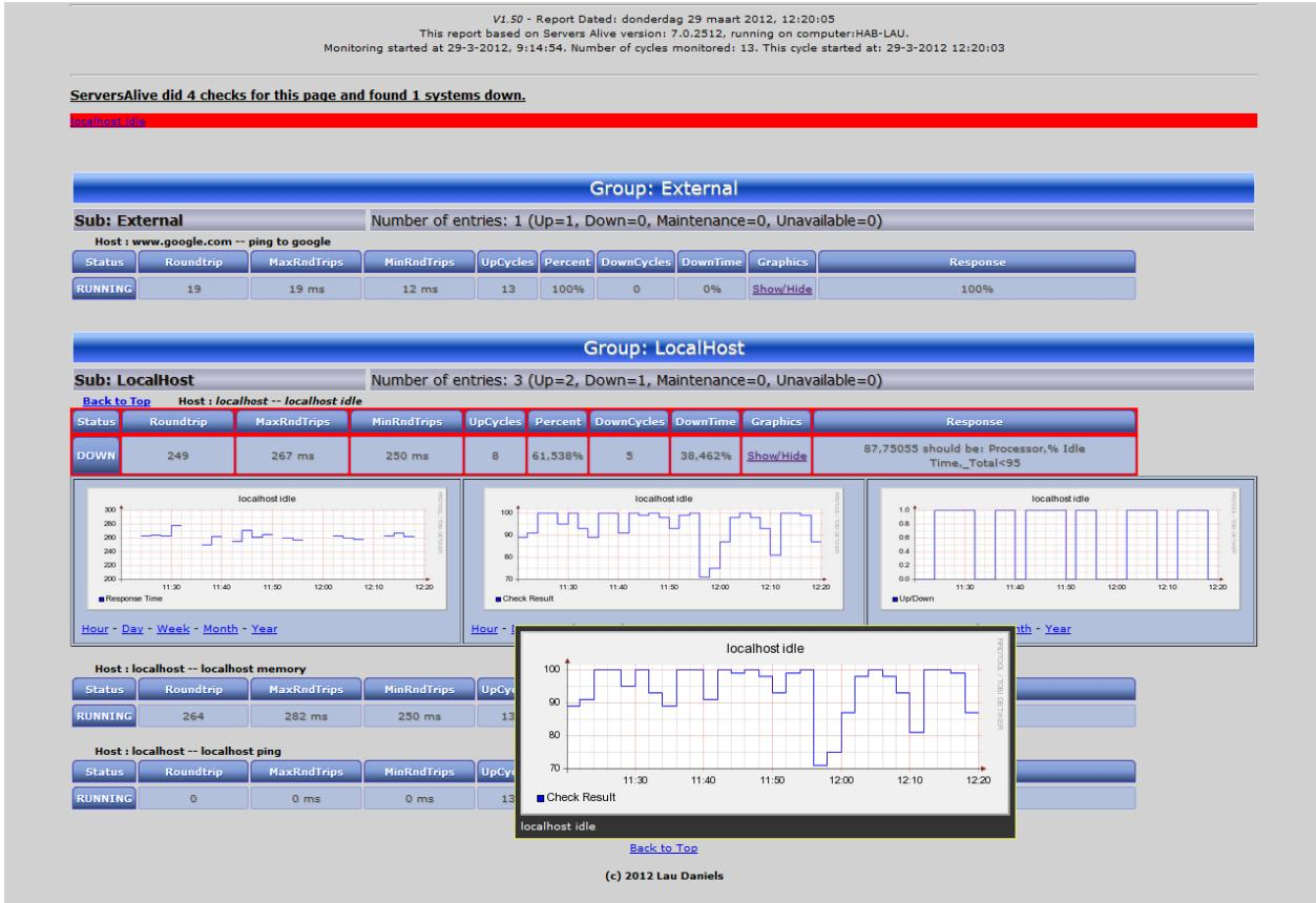
Notice that the roundtrip response time has gaps in the graph. When a system is down there is no response time recorded.
