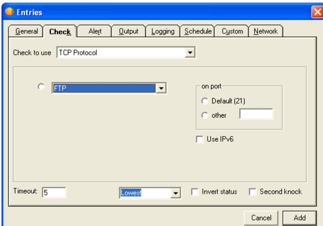
After supplying the needed information for the **General** tab of the **Entries** dialog box, you must select what type of check to use for the entry on the **Checks** tab. You can choose from many check options.
