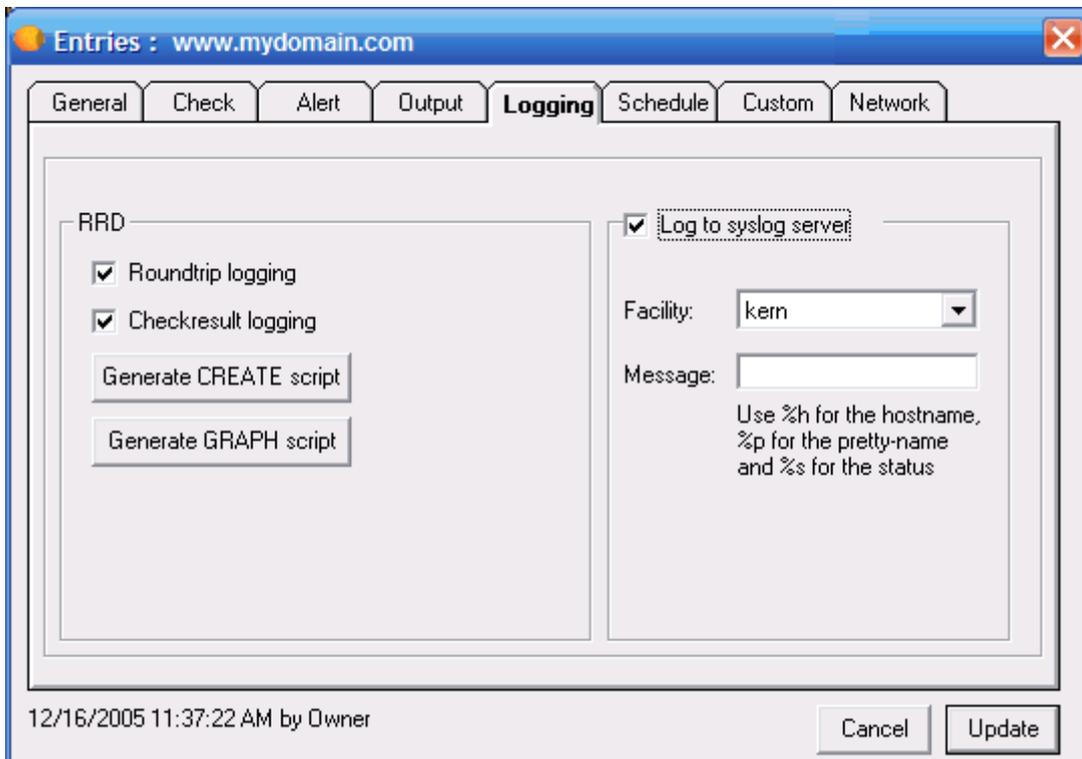
If you want to collect all of the up/down events that Servers Alive detects into a centralized logging server, you can use the settings on this tab. Syslog is a standard method of sending alerts to an alerting server. Free server implementations exist for both Windows and UNIX platforms.
