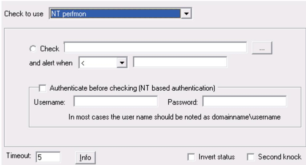
Servers Alive can perform various checks specific to Windows NT , 2000, and 2003. It can check NT performance monitor (perfmon) counters on local and remote computers. If you are running Servers Alive as a service, and want to check a service, process, or performance counter on a remote computer, you must specify a user name and password with sufficient rights to perform the check on the remote computer.
