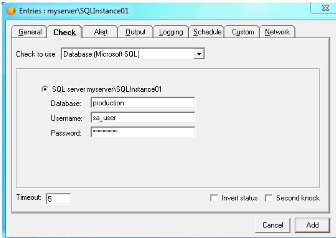
Servers Alive can check the availability of a Microsoft SQL Server database. To perform this check, the software uses the SMO object which must be installed separately. They can be found within the SQL Server PowerPack; you will need both the ENU\x86\SharedManagementObjects.msi and the ENU\x86\SQLSysClrTypes.msi files to be installed.
