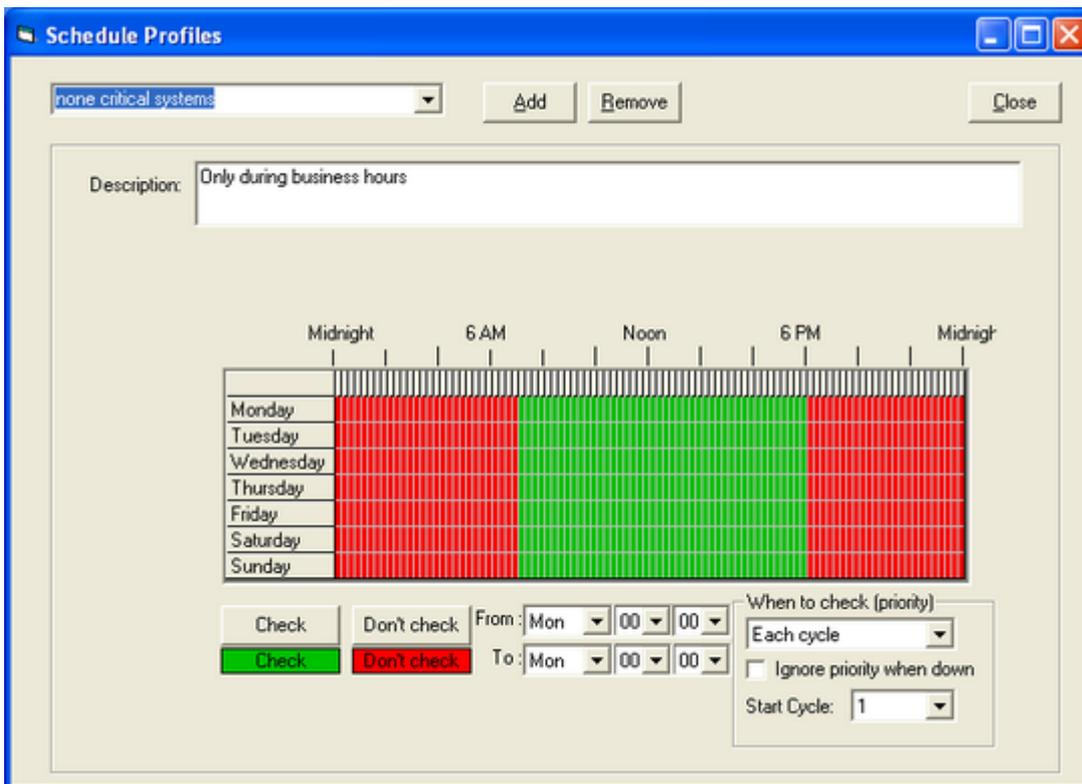
Many servers have a designated period of time during the week when they are unavailable. These are generally times for scheduled maintenance or backups. Instead of manually changing each host into maintenance mode every time the host needs to go into maintenance services, you can set up a schedule to tell Servers Alive when it should start and stop checking a host. You do this with the **Schedule** tab.
